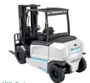
MXL Series Pneumatic Tire Models 80 Volt/AC-Powered Load Capacity (Ibs): 9,000 / 10,000 / 11,000 / 12,000
