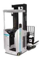
SRX Series Reach Truck Models 36V Single Reach Load Capacity (lbs): 3,500 / 4,500\*
